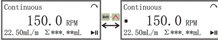
( 4 ) Press **Shift** + **Unit** to switch between speed and flow rate.
