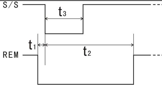
S/S—Start/stop signal; REM—bottle signal;  $t_1$ —Lead time of bottle signal;  $t_2$ —bottle signal duration;  $t_3$ —start signal duration
