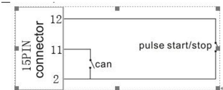
**Note:** ① Connection of pins 2 and 11 means “bottle available” and disconnection means “no bottle available”. A momentary contact of pins 2 and 12 means SS signal being received.
