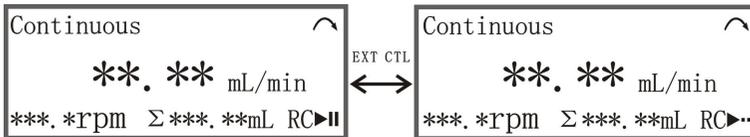
**Note:**When pump is controlled by external signal, users can press
