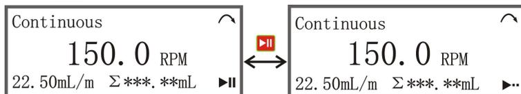
When “ReStart= ON”, turn the pump on, it will remain the same status with what it is before shut down.
