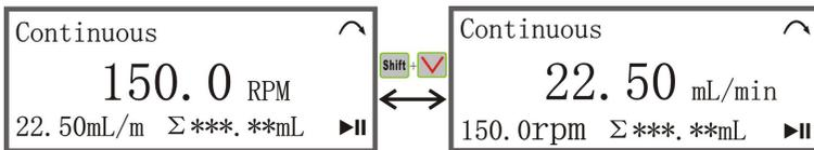
( 5 ) When pump stops, users can press **Shift** + **Max** to reset the cumulative volume to 0.
