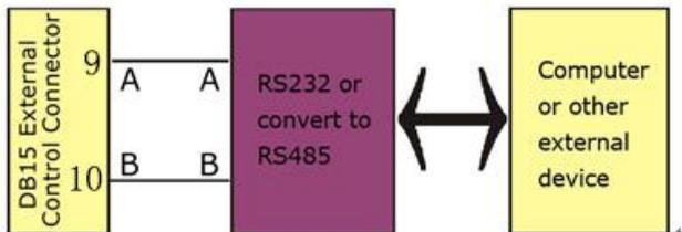
Remote communication control of multiple peristaltic pumps is needed in some applications. The 6/9 pins (A) and 7/10 pins (B) of the external control interface can be connected out according to Wiring 4 above to form the control system as shown in the figure below
